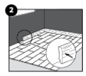
Inspect the final surface of the installed floor. Install vinyl skirtings against the wall but never attach the skirting to the floor itself. This method allows the floor to expand and/or contract under the skirting-
