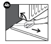
When sawing the panels make sure that the expansion gap under the door is 8mm. If you cannot lift the panel (e.g. under radiators), use the tapping block or pull-bar to tap the
