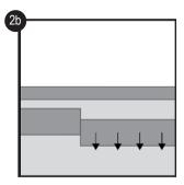
Slide one panel forward. Never fold up a panel, as this damage the profile.
