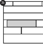
Apply glue on the cut groove side to adhere to the adjacent planks. When replacing planks the new plank will look different from the existing plank by the bevel size, texture, color, size and gloss level. There is color varies from batch to batch.
