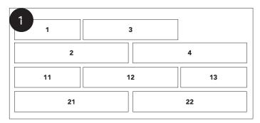
ESTABLISH STAGGER AND ALIGN TOOLS Products should be staggered in bricklaid pattern, stagger equal to half of a plank.
