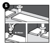
In rows where there is a pipe, make sure the pipe falls exactly in line with the short side of two planks. Take a drill bit with the same diameter as the pipe plus 16mm (0,63inch). Click the planks together on the short side and drill a hole centered on the joint between the
