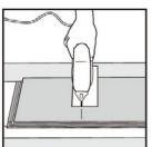
If cutting with a jig saw, the laminate surface should be turned down. If cutting with a hand saw, the laminate surface should be face up.
