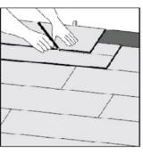
Step 6 Measure and cut final row of planks allowing for 3/8" expansion gap
