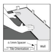
Step 1 Laying first plank in corner of room with tongue side facing wall using 3/8" spaces
