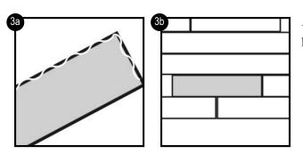
Apply glue on the cut groove side to adhere to the adjacent planks.
