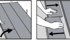
When installing each new row, take a Separate the whole row by lifting it up full loose plank and use the long side delicately at an angle. To separate the to tap against the prior row to ensure planks, leave them flat on the ground and slide them apart.
