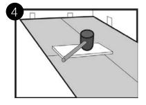
Afterwards use a tapping block and rubber mallet along both short ends to engage the planks. Place the tapping block over both short end and tap it with the mallet till the ends are engaged. Please be careful not to damage the profile or edges while engaging the planks. Test each plank before proceeding to the next row to make sure they are fully engaged.
