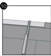
Last row (and perhaps also first row). Minimum width 50 mm. Place a spacer to the wall before measuring. Cut the panels lengthwise.
