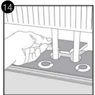
Fig 13 and 14. Installation at radiators. Drill the holes 2 x spacer thickness larger, than the diameter of the pipes.
