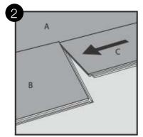
Second plank, first row. Place this plank (C) gently close to the short end of the first one (B).
