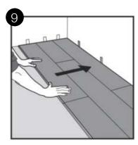
After 2-3 rows. Adjust the distance to the front wall by placing 10mm spacers.
