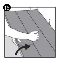
Separate the whole row by carefully lifting up and release the whole row. Fold up the row and release the whole long side.
