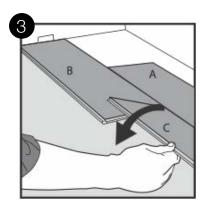
Fold it down with a single action movement. During the fold down, make sure the panels are close to each other.
