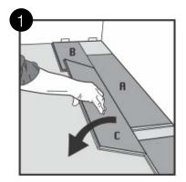
First row. Place a panel (A) as support for long side alignment of panel (B) and (C) while you install panel (B) and panel (C). Place a 10mm spacer between panel (B) and the wall. After that the complete first row is installed, remove panel (A) and slide the first row up against the wall with 10mm spacers placed between the panels and the wall. Later, after 3 rows, you can easily position the flooring against the front wall with predicted spacers.
