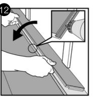
Fig 11 and fig 12. Cut off the vertical locking part of the strip with a chisel, put applicable glue on the strip and push the planks horizontally together. If necessary place some spacers between last board and the wall during the hardening.
